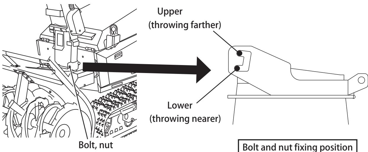
**Bolt and nut fixing position**
