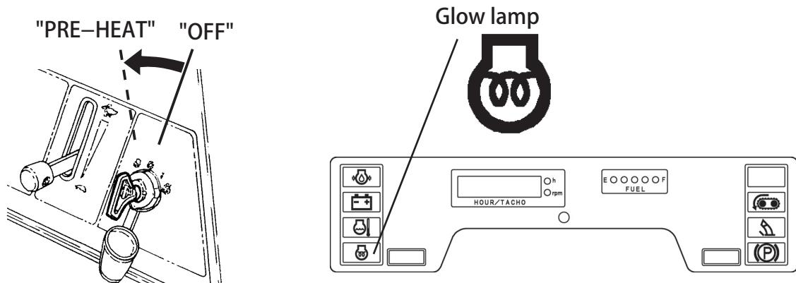
8. Turn the engine switch key.
