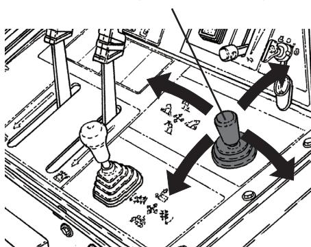
Auger housing adjustment lever
