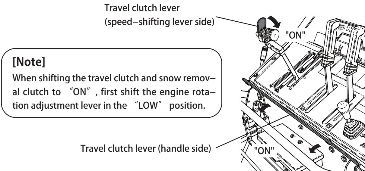
6 ) Set the snow removal clutch switch to “ON” . (Continue to press until the switch begins flashing.)
